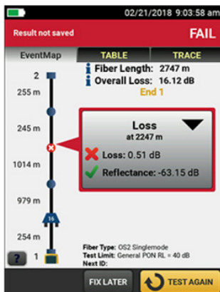
Link with an APC connector shown as a loss event
